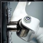
alloy spacers for vertical adjustment of chassis ( $\pm 13$  mm)
