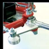
steering arm made of high-grade alloy steel
